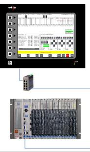
The **Optigalv**<sup>®</sup> system is composed of a touch panel (**HMI**), a programmable logic controler (**PLC**), an Ethernet network for data communication and connection to your local area network (LAN). The PLC reads/writes your plant analog and digital inputs/outputs (I/O) either by direct wired connections or via a fieldbus network (Profibus). Our software solution is integrated woth in the HMI and the PLC.
