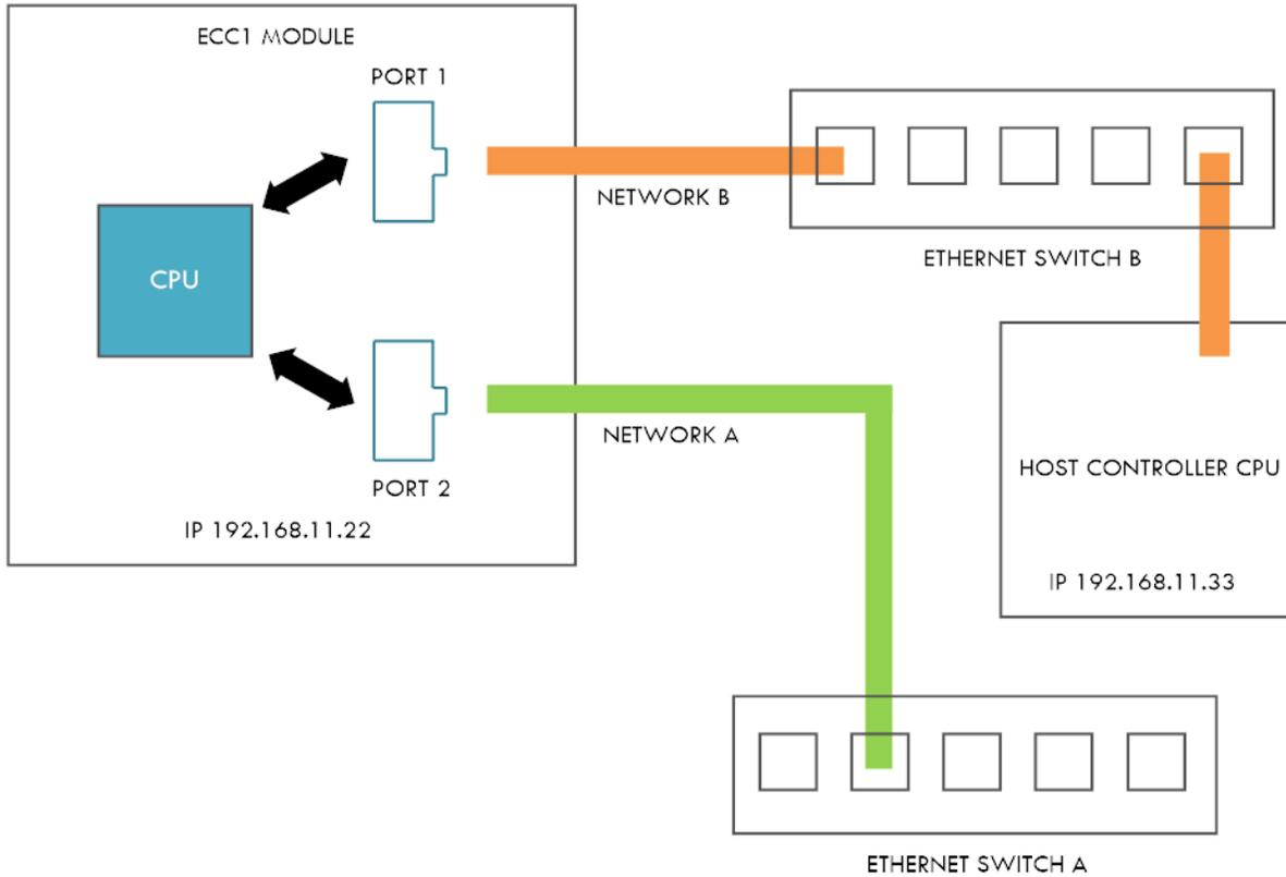
In this configuration the 2 networks connected to port 1 and port 2 are independent.
