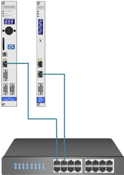
Using this method, all communications between the HMI and the 2500P-ECC1 module and between the 2500P-ECC1 module and the 2500 Series® controller pass through the network switch. In addition, communications between the programming workstation and the 2500 Series® controller pass through the network switch.
