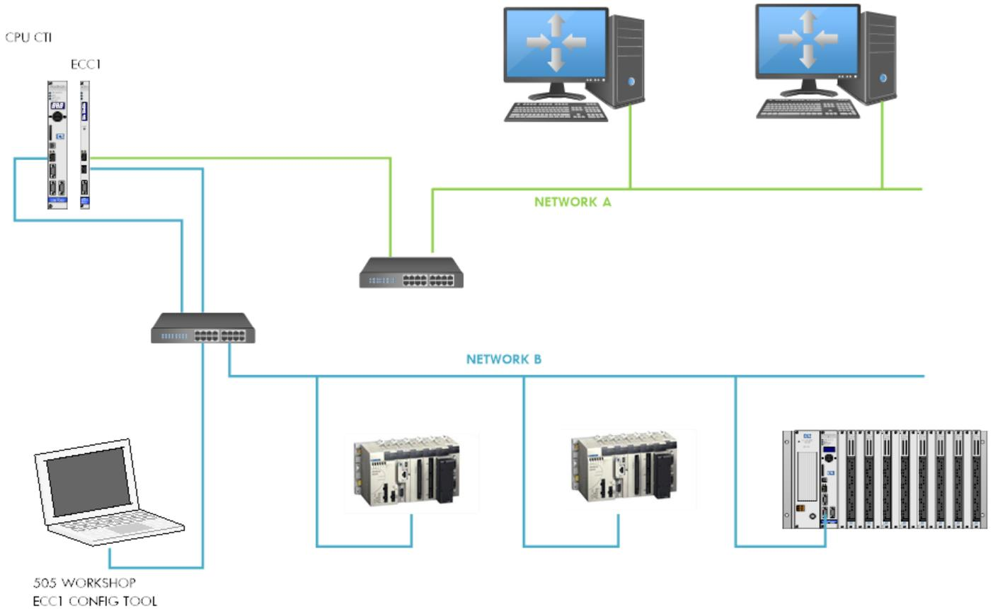
Network A is used to connect SCADA or HMI systems. Typically these systems would communicate to the ECC1 module. They would be configured to communicate to the IP address of the ECC1 module and would take benefit of the enhanced communication capabilities of the ECC1 module, which produces high update rates for the variables used on the SCADA system.
