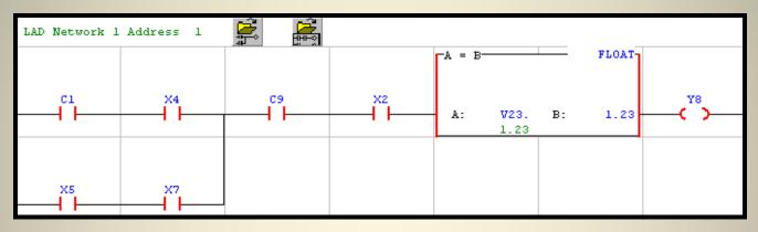
Equal To Floating Point Compare instruction in a ladder logic network
