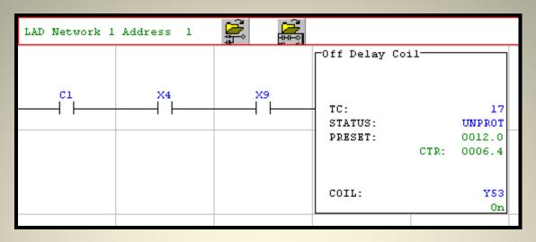
Off Delay Coil in a ladder logic network
