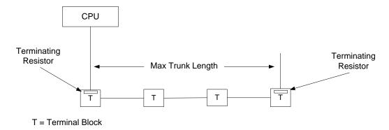
Figure 6. Trunk Length Measurement
