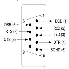
Figure 3. RS232 Serial Port
