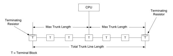
Figure 7. T-Connection Trunk Length
