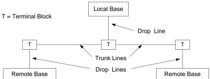
Figure 5. Remote I/O Installation
