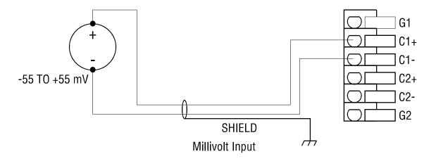
Figure 18 Millivolt Wiring Application
