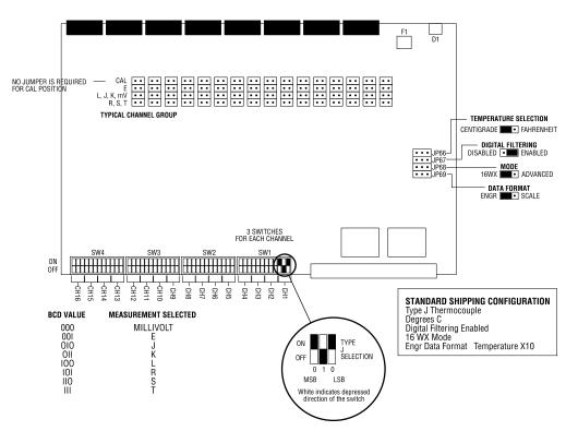
Figure 15 Configuration Jumper Location
