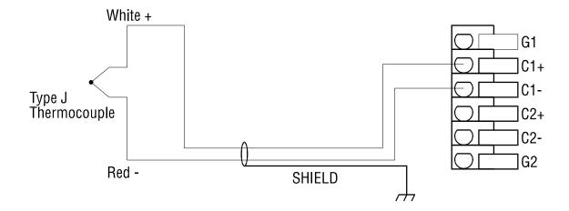
Figure 17 Thermocouple Wiring Application
