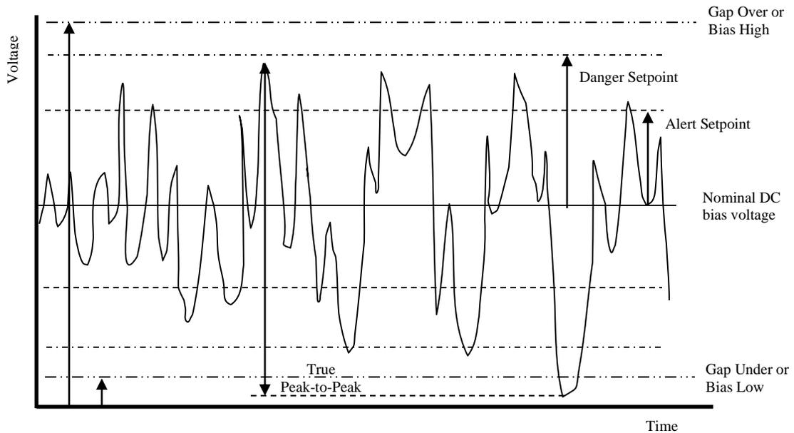
Figure 3.1. Alarm & Danger levels, Time Delay example chart
