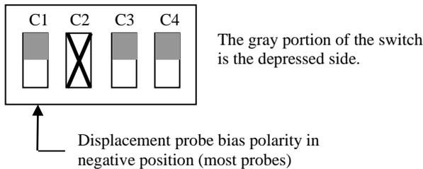
Note: Switch C2 is not read if a displacement probe is used. If the displacement probe requires positive bias, set C1 to the “down” position (relative to the backplane of the board). C3 and C4 must be in the “up” position.
