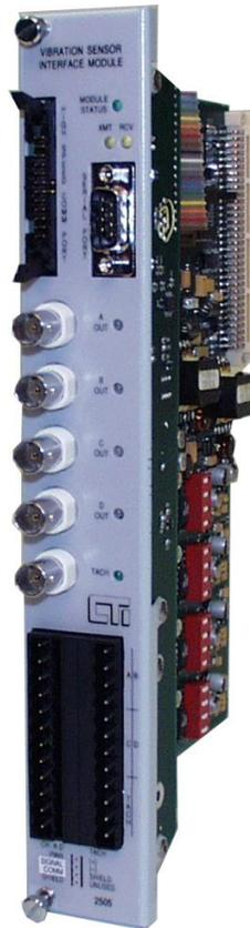
**The 2505 4-Channel Vibration Sensor Interface Module**
