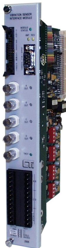
**The 2505 4-Channel Vibration Sensor Interface Module**
