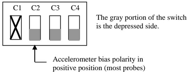
Note: Switch C1 is not read if an accelerometer is used. If the accelerometer requires negative bias, set C2 to the “up” position (relative to the backplane of the board). C3 and C4 must be in the “down” position.
