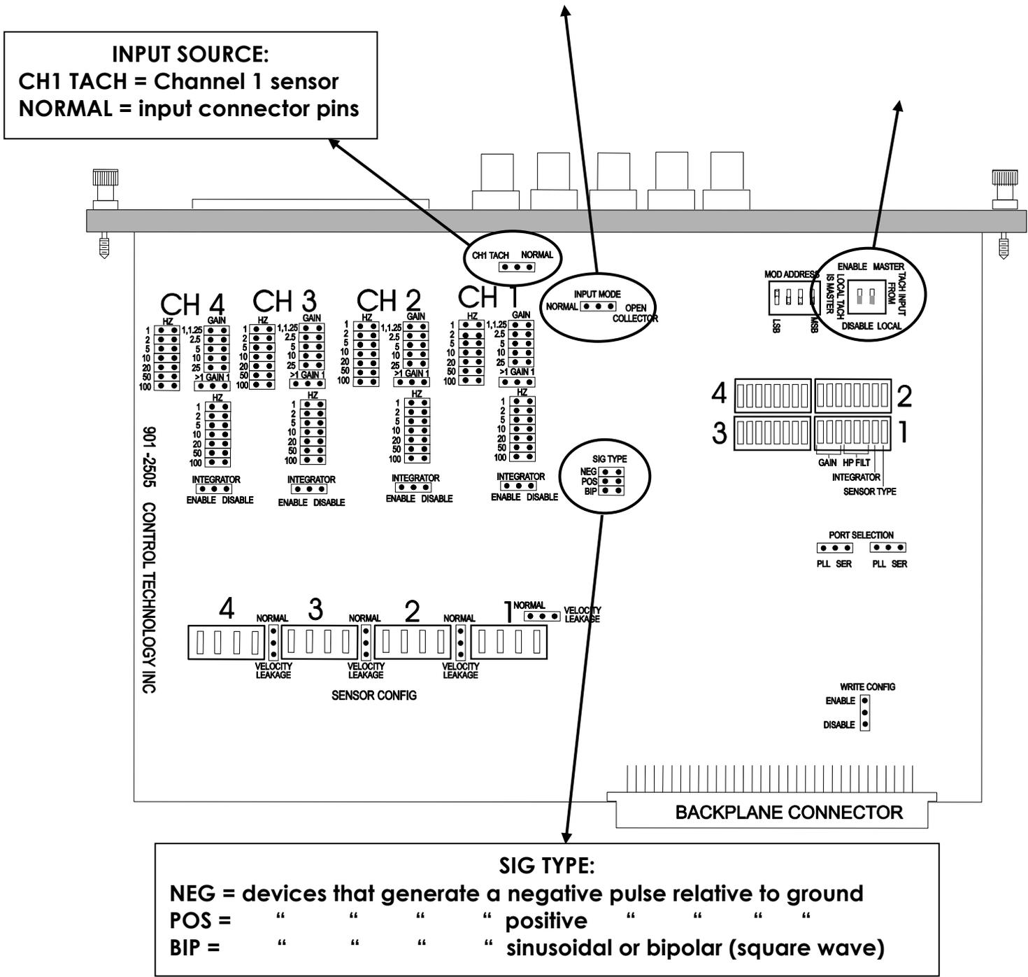
Figure 2.7. Selecting Tachometer Options
