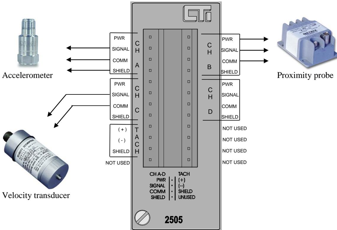
Figure 1.1.a. CTI 2505 Wiring Connector
