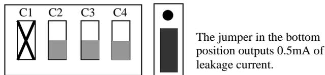
The jumper for Channel 1 is located above the switchblock; the left position is NORMAL and the right position is LEAKAGE CURRENT.
