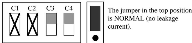
Note: Switches C1 and C2 are not read if a velocity probe is used. The internal circuitry reads the probe as a displacement probe without bias voltage. C3 and C4 must be in the “up” position.
