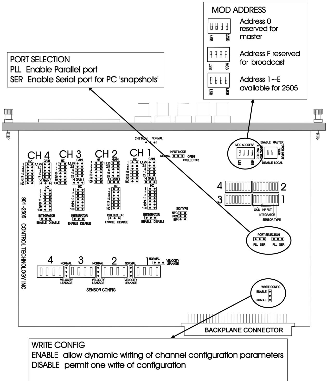
Figure 2.8. Selecting the Port Type, Module Address, and Write Configuration
