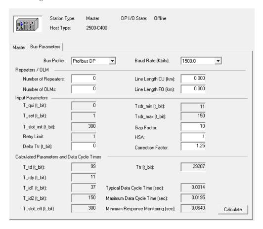
The Bus Profile **Profibus DP** sets default parameters on the bus, while allowing you to specify parameters such as Baud Rate, the number of repeaters and OLMs, and bus line length. This profile conforms to EN 50170, Volume 2, PROFIBUS standards, and in most cases will provide the best performance for your Profibus system. The **Adjustable** profile allows you to configure all bus parameters. Each parameter and its function is listed below.
