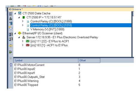
Repeat this process to populate the variables of "STATUS" through "TripLog4" to the Write to V-Memory block (third block). Do a renumber. The result should look like this:
