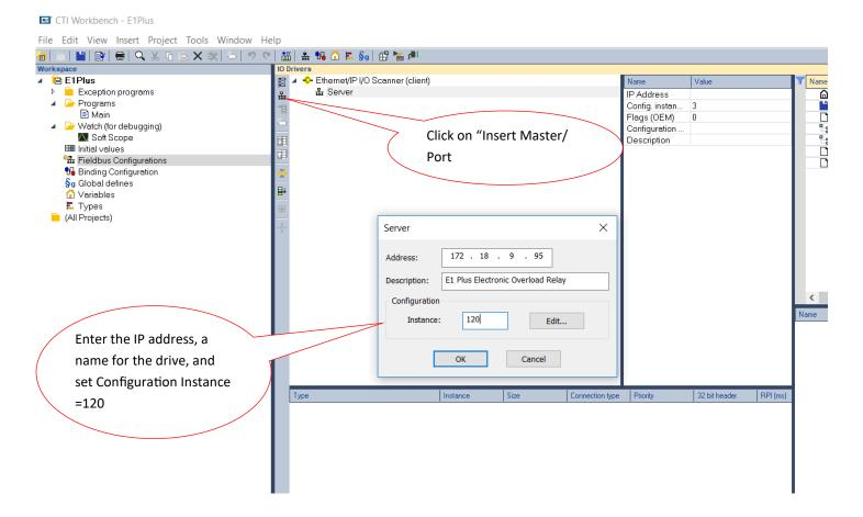
6. Set the Connection Parameters. I/O data is accessed using Input Instances 50, 51, 106, 110 or 111 and Output Instances 2, 101 or 103. The size of the input connection and the output connection shall correspond to the size of the chosen instance. The E1 Plus configuration assembly instance is 120. In this example configuration data is not used, so the data size is set to 0.
