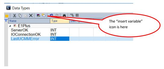
Referring to Table 22 and Table 17 on page 10, add all the other E1Plus parameters, first from Table 17 then from Table 22. "Output I/O" list, then from the "Input I/O—Generic" list. Set the type for each as shown below. Put a description if you want. Close the Data Type window when finished.
