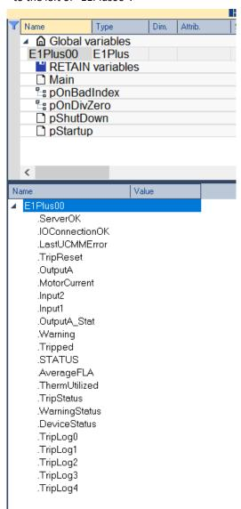
We will use this list to drag variable names over to our Ethernet/IP connections. First, drag the three driver variables (one at a time over to their corresponding locations in the "Drive to E1Plus" connection.
