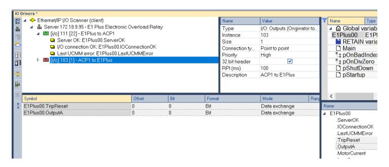
For the E1Plus00.TripReset variable, double-click in the "bit" column and change the bit from 0 to 2, since this is bit 2 in byte 0 (see Table 17 on page 10).
