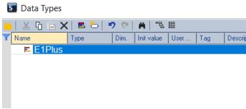
Now we will add the elements to the structure. Use the "Insert Variable" icon to add each element. First add the driver variable names which will be tied later to the driver variables. Set each type to "INT" (integer).
