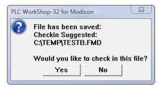
Clicking **Yes** displays the Check In dialog box. After the file is checked in, PLC WorkShop for Modicon keeps the file checked out to you so that you may continue editing the program. Clicking **No** saves the working copy on your computer but does not write any changes to the FTVersionTrak repository. The file can be checked in manually by clicking on the FTVersionTrak toolbar.
