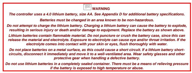
The Janus controller monitors battery status and provides 'Battery Low' indication when the battery has approximately 30% of its usable life remaining. At this point, the battery will still provide adequate power for power-loss conditions for some period of time (based on size of application and number of occurrences). However, a replacement battery should be ordered and installed as soon as possible.
