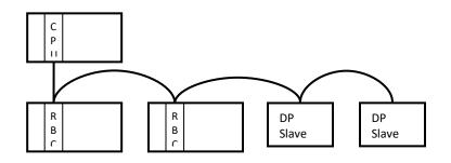
Up to 32 devices can be connected on a single segment. To increase distance or the number of devices supported, segments can be interconnected by using repeaters. Up to 10 segments may be connected together.
