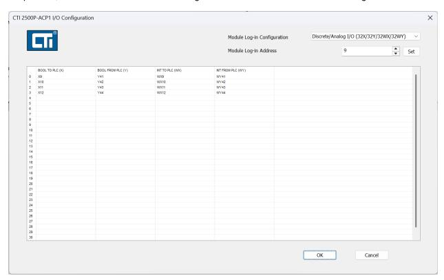
In this configuration, the user had specified that the ACP1 would log in to the base at address 9. Accordingly, the I/O available in the interface was:
