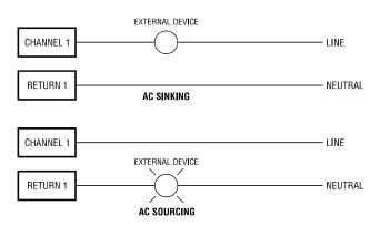
Fig 2. Typical External Wiring Application 2590-EF
