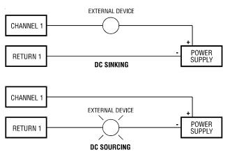
Fig 5. Typical External Wiring Application 2591-EF
