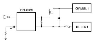
Fig 4. Typical Internal Circuit - 2591-EF
