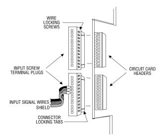
Figure 20 Input Connector Wiring
