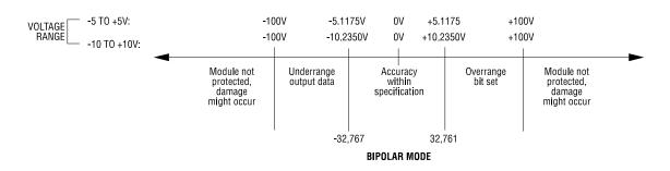
Figure 11 Voltage Input Limits (Bipolar)
