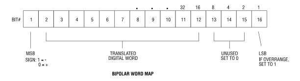
Figure 4 Word Input to the PLC from the Module (Bipolar)
