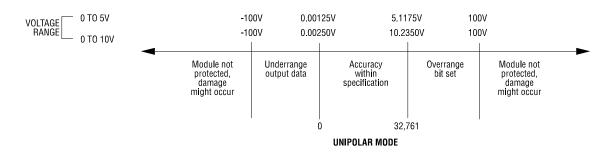
Figure 10 Voltage Input Limits (Unipolar)
