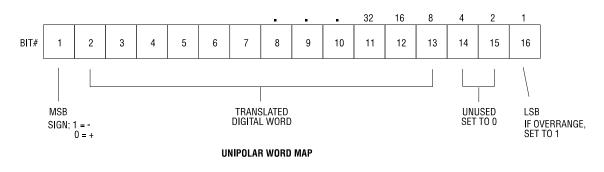
Figure 3 Word Input to the PLC from the Module (Unipolar)
