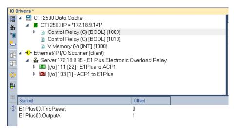
Now highlight the "Write to Control Relay" block (the second block). From the variable list at the right, highlight the variables ".MotorCurrent" through ".Tripped". Drag these into the box below the fieldbus configurations. Do a renumber as we did in the previous step. The result should look like this:
