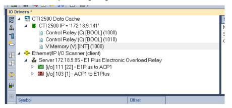
Now we will use the same "drag and drop" procedure we used in step 12, to populate the variables read from / written to the PLC. First highlight the "Read from Control Relay" block (the first block). From the variable list at the right, highlight the variables ".TripReset" and ".OutputA". Drag these into the box below the fieldbus configurations:
