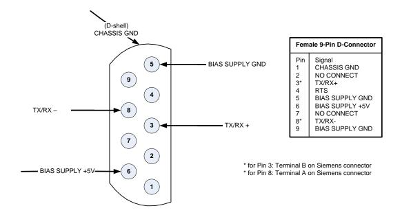
Figure 5. Profibus Female DB9 PIN Out Diagram
