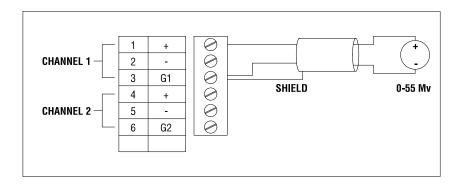
Figure 10 : Millivolt Wiring Application
