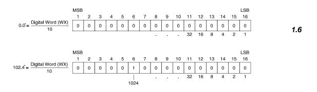
Figure 3: Example Change in Input Level
