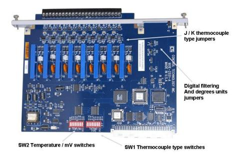
Figure 7 Setup Jumpers and Switches
