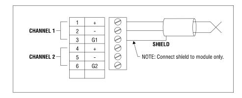
Figure 9 : Thermocouple Wiring Application
