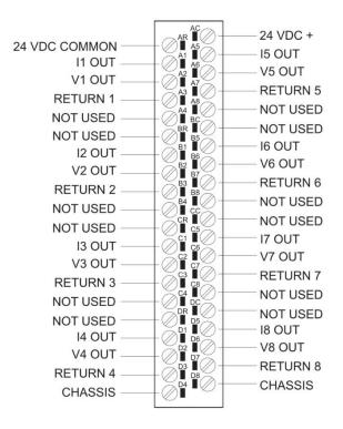
Figure 6 Output Screw Terminal Plug Wiring
