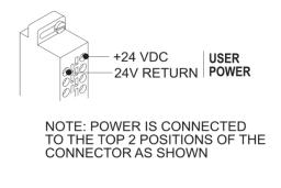
**Figure 9 Power Supply Connection**
