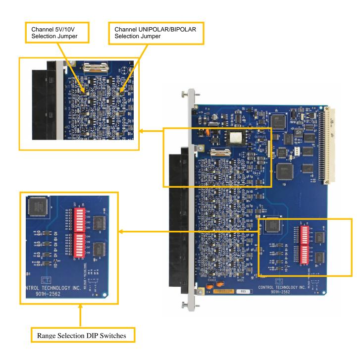
**Figure 4 Channel Voltage and Range Selection**
