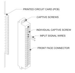
Figure 8 Attaching the Screw Terminal Plug
