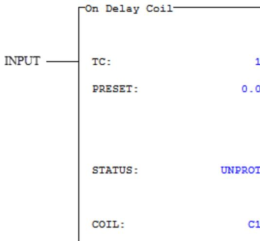
The On Delay Coil instruction is only compatible with the CTI 2500 family of processors. It requires a CPU firmware of V6.18 or later.
