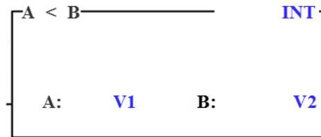
When the input is energized, the LESS instruction compares two integers, two unsigned integers, or two floating point values, and energizes the output if, and only if, the first value (**A**) is less than the second value (**B**).
