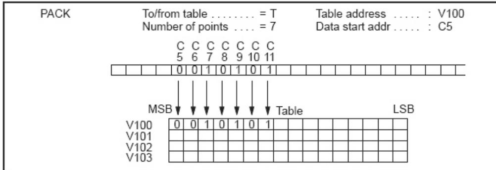
Figure 11 – Example of PACKing Bits To a Table
