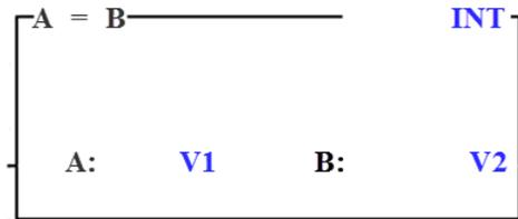
When the input is energized, the EQU instruction compares two integers, two unsigned integers, or two floating point values, and energizes the output if, and only if, the first value (**A**) is equal to the second value (**B**).
