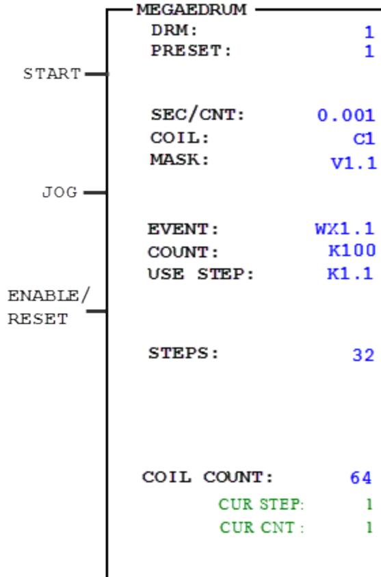
The Mega Time/Event Driven Drum (MegaEDRUM) instruction is only compatible with the CTI 2500 family of processors. It requires a CPU firmware of V6.18 or later. It is similar to the EDRUM instruction, but the MegaEDRUM supports more steps and coils. The MegaEDRUM supports up to 128 coils (horizontally) and 128 steps vertically. The EDRUM instruction is limited to 15 coils (horizontally) and 16 steps (vertically).
