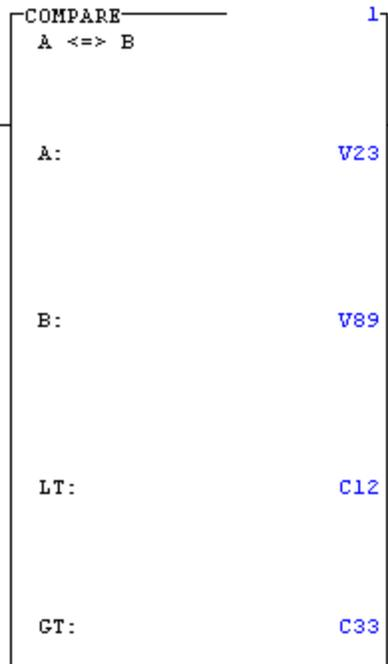
The Compare instruction (CMP) compares a signed integer value in A with a signed integer value in B. Based upon the comparison, the coil or relay addresses may be turned on or off.
