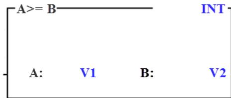
When the input is energized, the GEQ instruction compares two integers, two unsigned integers, or two floating point values, and energizes the output if, and only if, the first value (**A**) is greater than or equal to the second value (**B**).
