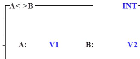
When the input is energized, the NEQ instruction compares two integers, two unsigned integers, or two floating point values, and energizes the output if, and only if, the values are not equal.
