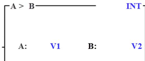
When the input is energized, the GTR instruction compares two integers, two unsigned integers, or two floating point values, and energizes the output if, and only if, the first value (**A**) is greater than or equal to the second value (**B**).
