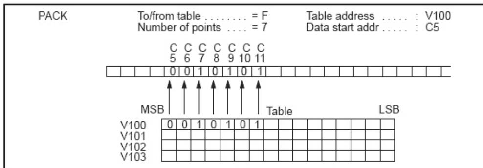
Figure 14 – Example of PACKing Bits From a Table
