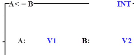
When the input is energized, the LEQ instruction compares two integers, two unsigned integers, or two floating point values, and energizes the output if, and only if, the first is value (**A**) less than or equal to the second value (**B**).
