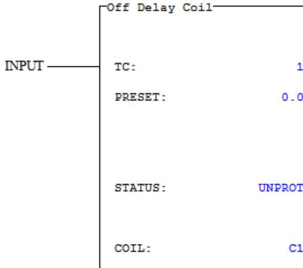
The Off Delay Coil instruction is only compatible with the CTI 2500 family of processors. It requires a CPU firmware of V6.18 or later.
