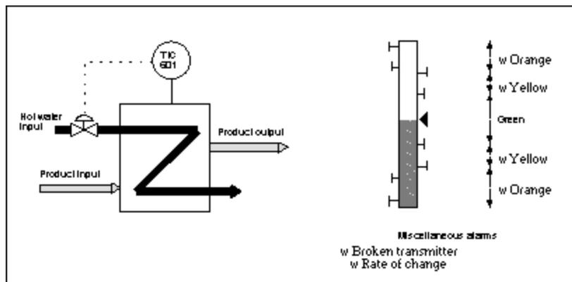
The high-high, high, low, and low-low alarms are fixed absolute alarms and may correspond to warnings and shutdown limits for the process equipment itself. The yellow and orange deviation alarms move up and down with the setpoint, and may refer to specification tolerances around the setpoint.
