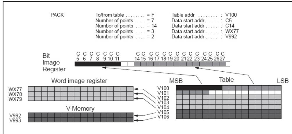
Figure 17 – Example of PACKing Bits and Words From a Table
