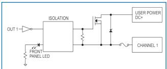
Figure 2. Typical External Wiring Diagram
