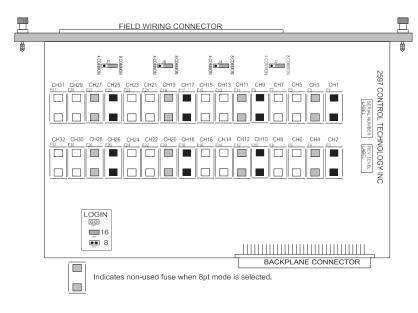
Figure 1. Jumper and Fuse Configuration
