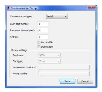
4. In **Communication Type**, select **Serial** to connect to a PLC using serial communication; select **TCP/IP** to connect to a PLC/Ethernet adapter using TCP/IP.
