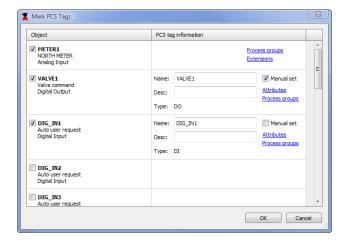
In the Mark PCS tags dialog box, the objects named METER1, VALVE1, and DIG\_IN1 are all marked for translation. For the VALVE1 and DIG\_IN1 objects, you can type a new name for the PCS tag in the Name box and a description for the PCS tag in the Desc box.
