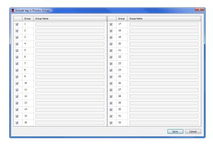
In the **Include tag in Process Groups** dialog box, the check boxes associated with the groups where the tag will be included are selected. By default, all tags are initially assigned to all 32 process groups. To remove a tag from a process group, clear the check box. The **Include tag in Process Groups** dialog box is equivalent to the process groups sub-editor in APT.
