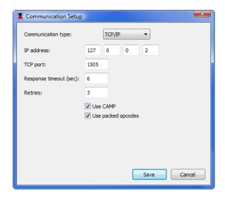
In the **IP Address** box, enter **127.0.0.1**. In the **TCP port** box, enter **1505** in the TCP Port box. The TCP Port must be set to 1505 to enable connection with the simulator. The other communication settings can be changed as needed; refer to the FTSolution for APT online help for additional information.
