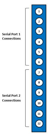
The pin-out (i.e. function for each serial port terminal) varies according to the specified electrical interface (RS232, RS422, or RS485). See APPENDIX D: Serial Port Wiring for the pin-out for each electrical interface.
