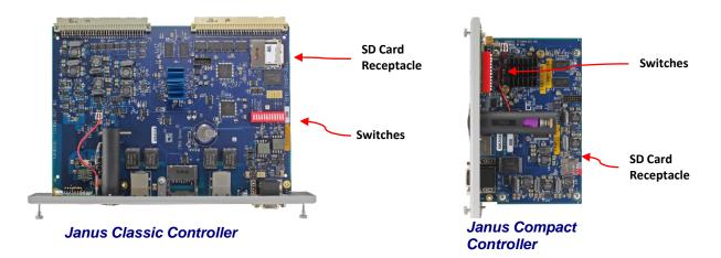
To remove and replace the internal SD card:
