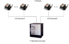
Figure 2: Existing Control System
