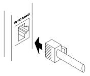
Insert the 8 pin (RJ-45) plug on your unshielded twisted pair cable into the RJ-45 jack on the 2572. Push the plug into the jack until the plug clicks into place.
