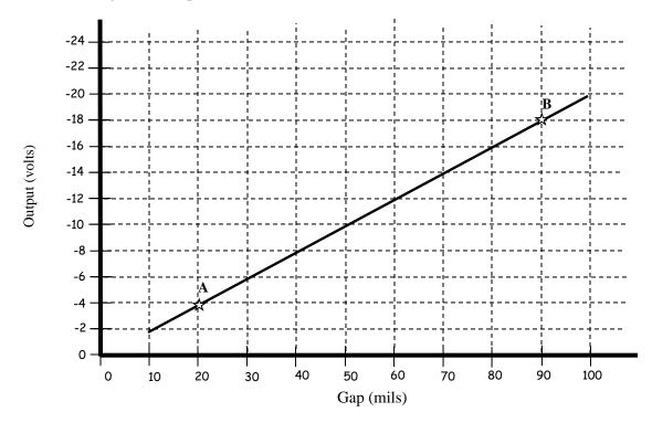
Figure 3.2. Displacement probe (200mV/mil) chart example
