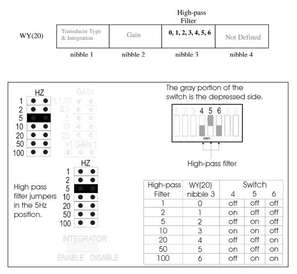
Figure 2.3. Selecting High-Pass Filter Value
