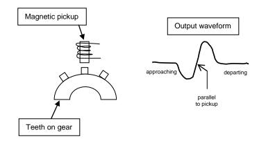
Figure 2.6. Bipolar gear tooth example
