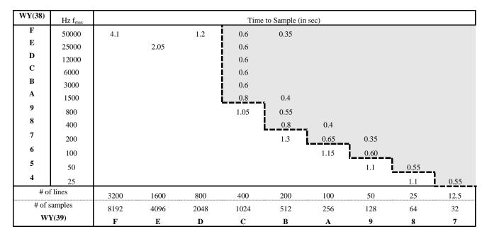
*Figure 3.3. Time to Sample Correlation Chart* (cells in the shaded area indicate API670-compliant region)
