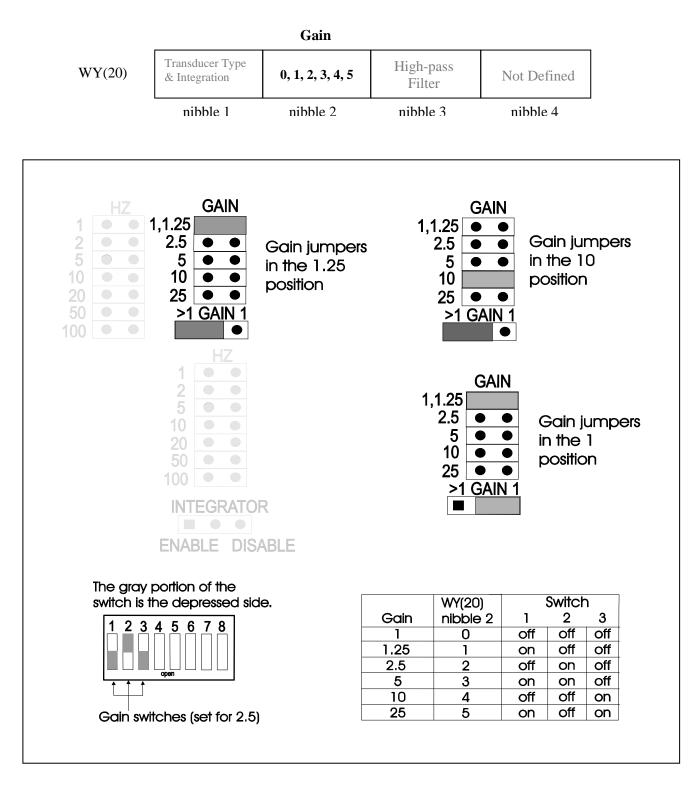
Figure 2.4. Selecting the Gain Range and Value
