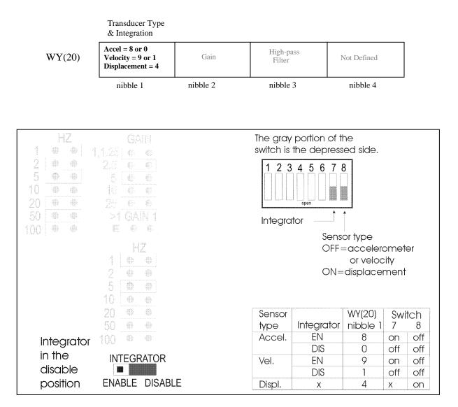
Figure 2.5. Selecting the Integration and Sensor Type
