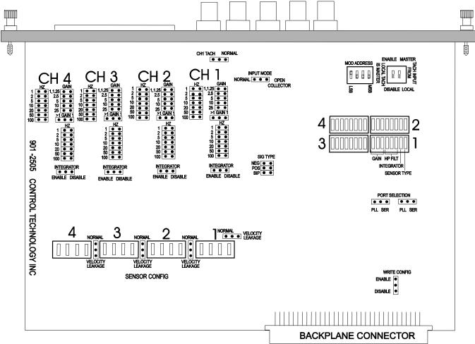
Figure 2.1. Jumper and Switch locations
