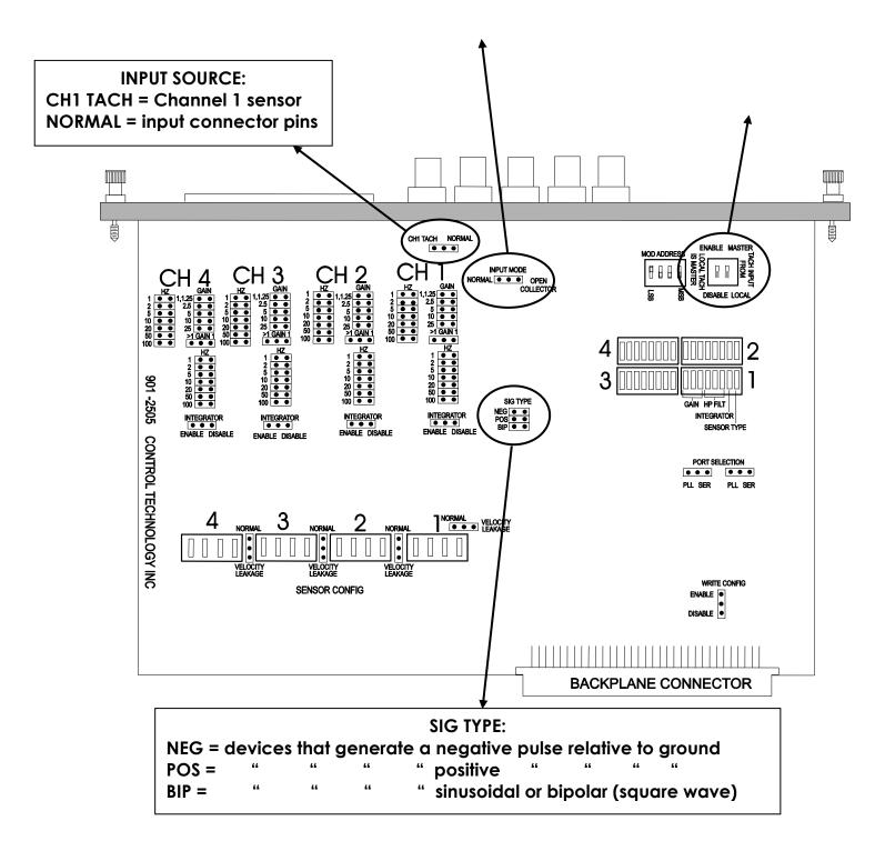
Figure 2.7. Selecting Tachometer Options
