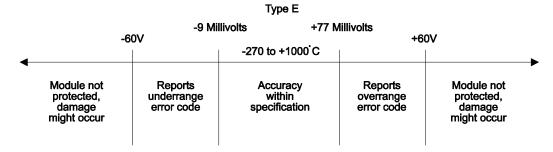
Figure 8 Effect of Voltage Input on Type E Thermocouple
