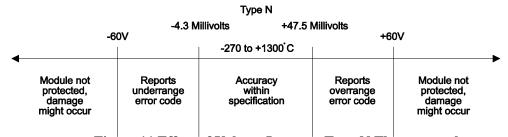
Figure 11 Effect of Voltage Input on Type N Thermocouple
