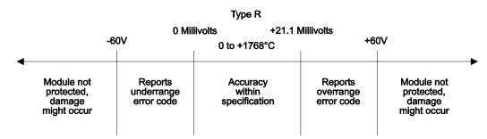
Figure 9 Effect of Voltage Input on Type R Thermocouple
