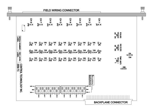
**Figure 16 Configuration Jumper Board Locations**
