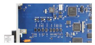
**Figure 19 Thermocouple Selection Jumpers**
