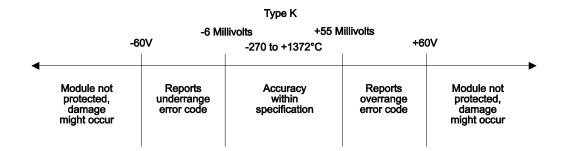
Figure 6 Effect of Voltage Input on Type K Thermocouple
