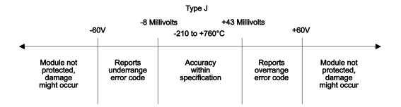
Figure 5 Effect of Voltage Input on Type J Thermocouple
