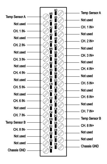
**Figure 21 Screw Terminal Connector Wiring**
