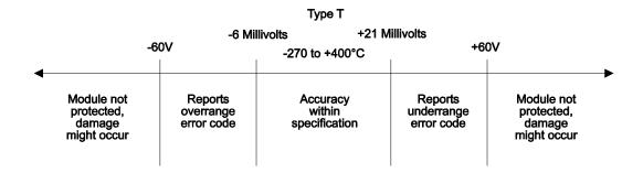
Figure 7 Effect of Voltage Input on Type T Thermocouple
