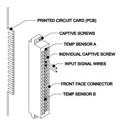
**Figure 26 Input Connector Assembly**
