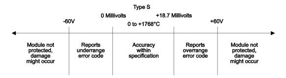
Figure 10 Effect of Voltage Input on Type S Thermocouple
