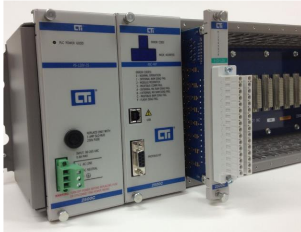
Figure 28 2500C-8-TC Module Physical Installation Picture
