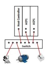
If you are connecting more than one CTI Advanced Function Module to the same Host PLC, you should make all Ethernet connections through an external Ethernet switch as shown in the figure on the left.
