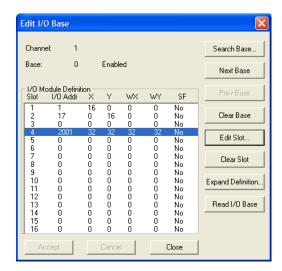
The Mixed I/O interface requires special care when assigning an I/O Address because the Series 505® model allows one "login" address for each module slot. Therefore, the I/O Address assigns the image register positions for both the Discrete I/O and Word I/O values.
