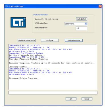
If an error occurs, an error status is returned to *CTI Workbench*. An error code is displayed on the module LED display (see *APPENDIX A: ERROR CODES*) and the firmware update process is terminated. The user must go to the module location to diagnose and correct the error condition.
