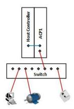
be placed in the same base as the Host PLC, the preferred Data Cache Interface connection is a short Ethernet cable (Cat 5 or Cat 5e) from one of the Ethernet ports on the 2500P-ACP1 to the Ethernet port on the 2500 Series® CPU. A second Ethernet cable is then connected from the other port to a network switch that provides a path to the other devices.
