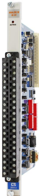
Figure 1 The Model 2555-A 16-Channel Differential Analog Input Module
