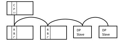
Up to 32 devices can be connected on a single segment. To increase distance or the number of devices supported, segments can be interconnected by using repeaters. Up to 10 segments may be connected together.
