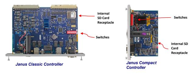
To remove and replace the internal SD card:
